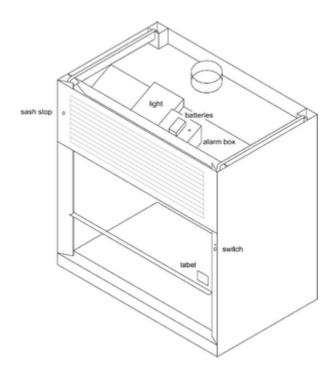
**The alarm box** is a grey plastic enclosure located on top of the fume chamber. Refer the diagram. The control box contains
