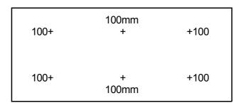
The average velocity (sash open) should be more than 0.5m/sec Measure the airflow
